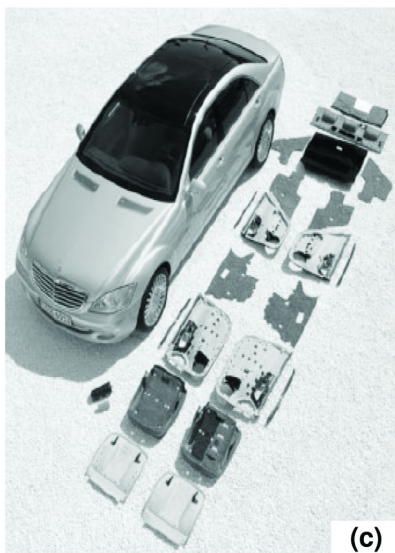
Figure 10. (a) Commercial BRC products in North American Market (b) BRC in building applications, (c) BRC automobile parts. (Reproduced with permission of (243). Copyright Wiley-VCH Verlag GmbH & Co. KGaA)
