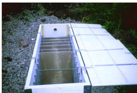
Figure 8. A nonwoven filtration system made of wood lignocellulose to remove heavy metals from contaminated water.
